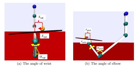
**Fig. 7.** Ball-balancing task using a Barrett WAM $^{\rm TM}$  arm simulator. Two joints of the robots are controlled so as to keep the ball in the middle of the tray.
